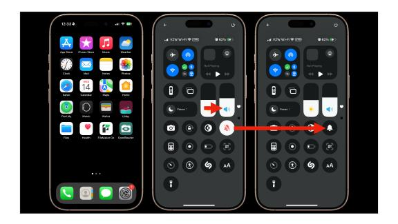
3. The **Control Center** has additional controls over the Volume of the iPhone. On the example screens above you can see the taller **Volume slider**, and below it I have placed the **Mute** control (Bell), which works as a toggle. Use these areas to adjust the volume of some sounds, but not all sounds are controlled by these areas. (More to come...)
