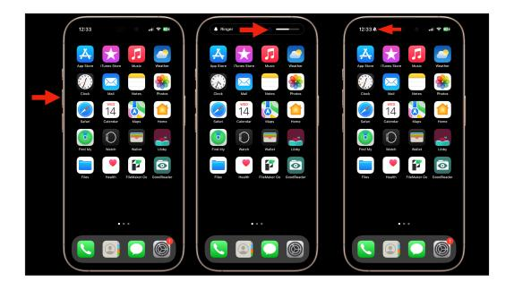
2. The Up and Down **Volume Buttons** on the left of the iPhone are just one of the places which can adjust your volume. Try pressing them while watching for an indicator at the top or left side of the screen to indicate how the volume is changing with each press.
